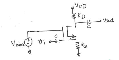
For Small signal Analysis, equivalent clocuit
