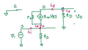
Voltage gain and input impedance
